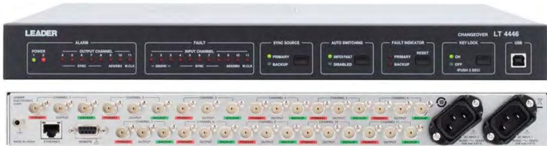
The LT4446 is a changeover unit that automatically switches the signal from the primary signal to the backup signal when problems are detected in the primary signal. Two systems of input signals (primary and backup) are connected to the LT4446. The changeover detects errors in the amplitude of the primary input signal.
