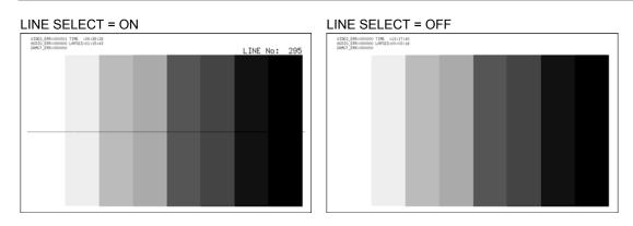
Figure 9-13 Turning line selection on and off
