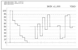
Figure 11-7 Displaying markers for 75 % intensity color bars
