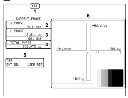
Figure 14-9 Phase difference measurement screen
