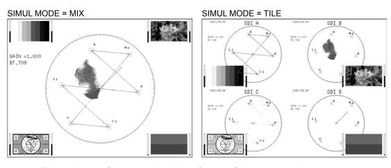
Figure 12-14 Selecting the display format of simultaneous input mode
