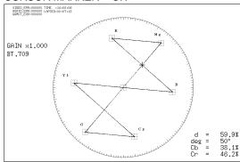
Figure 12-7 Displaying the vector marker
