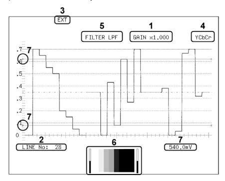
Figure 11-1 Video signal waveform display
