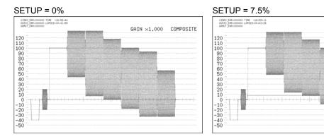
Figure 11-22 Selecting the setup level
