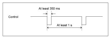
Figure 15-2 Control timing 1
