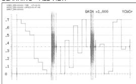
Figure 11-25 Displaying blanking intervals
