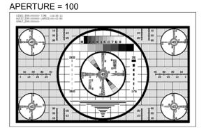
Figure 9-4 Setting the aperture
