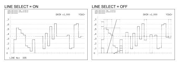
Figure 11-18 Turning line selection on and off
