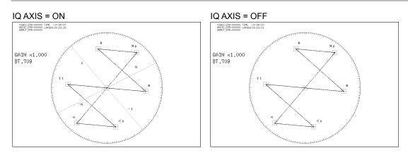
Figure 12-3 Turning the display of the I and Q axes on and off
