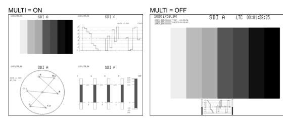
Figure 6-2 Switching between the single- and multi-screen displays
