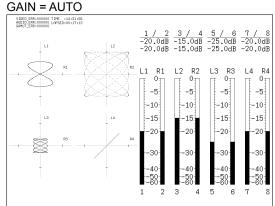
Figure 13-9 Lissajous curve gain
