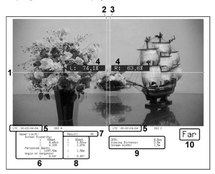
Figure 10-8 Disparity measurement display
