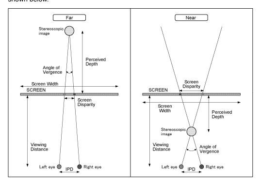
Figure 10-9 Setting and measurement item names
