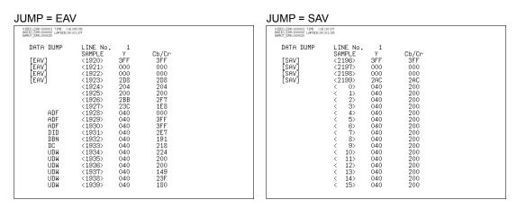
Figure 14-7 Selecting the display start position
