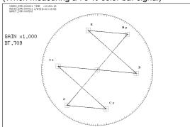
Figure 12-18 Displaying a scale for 75 % intensity color bars
