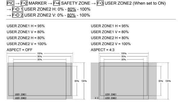
Figure 9-11 User marker setup examples
