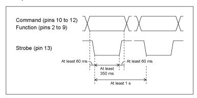
Figure 15-4 Control timing
