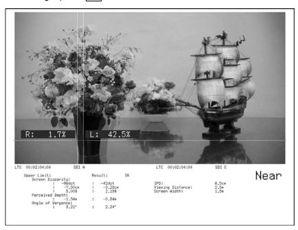
Figure 10-11 Disparity measurement display
