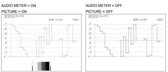
Figure 11-27 Setting the thumbnail display
