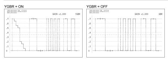
Figure 11-21 Displaying the luminance and GBR signals simultaneously
