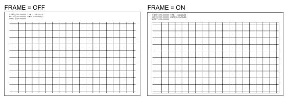
Figure 9-6 Turning the display of the frame marker on and off
