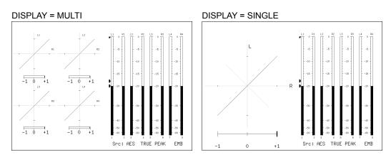
Figure 4-2 Selecting the Lissajous curve display format
