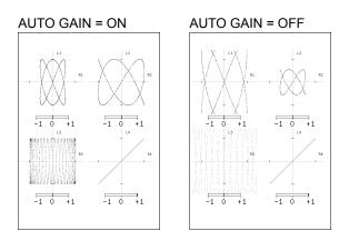
Figure 4-4 Setting the Lissajous curve gain
