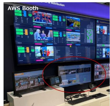
The NDI Checker introduced the technology of a software-based system that enables direct waveform monitoring in native NDI systems, which is becoming increasingly popular in the market.
