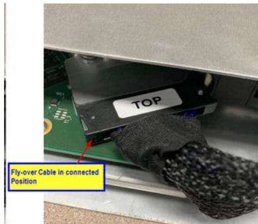
Figure 46: Reconnecting the Fly-over Cable
