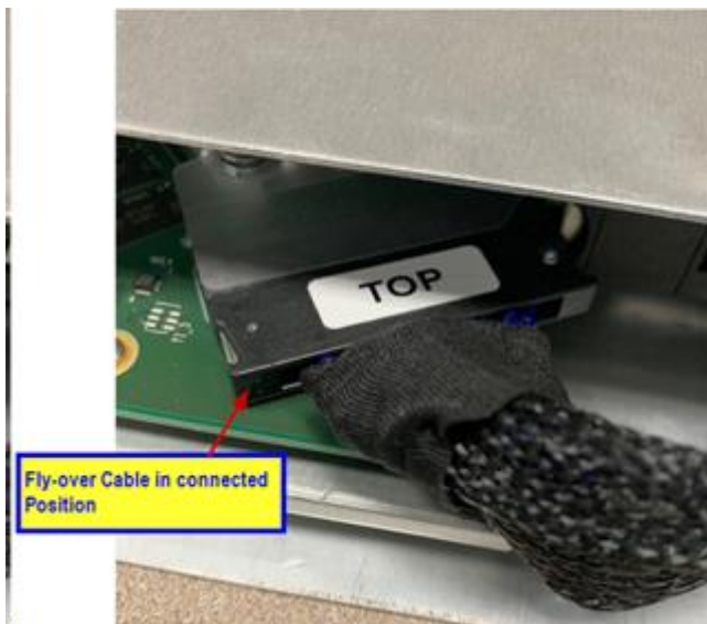
Figure 33: Reconnecting the Fly-over Cable
