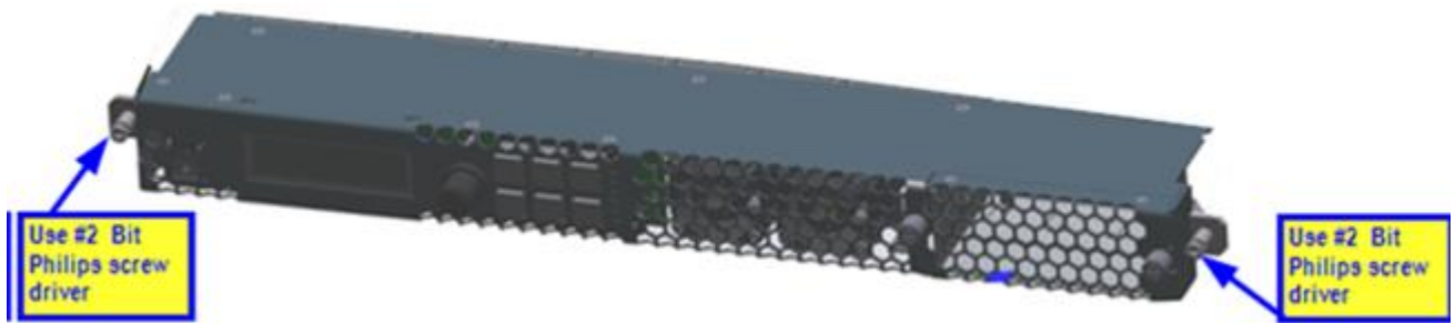
Figure 53: Secure the Front Panel with Screws
