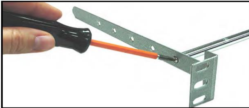
Figure 6: Attaching the Cable Relief Bar
