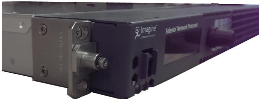
Figure 3: Mounting Ear on Front Panel
