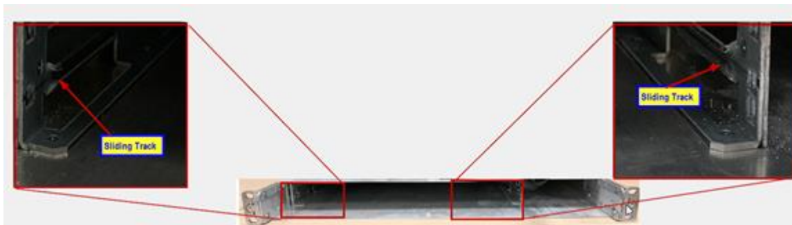
Figure 25: Sliding Track Positions
