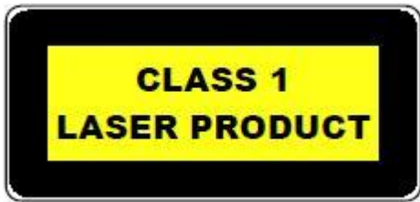
Figure 55: Label for Class 1 Laser Products
