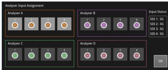
**Select All Source Inputs on All Analyzer to Compare Side-by-Side**
